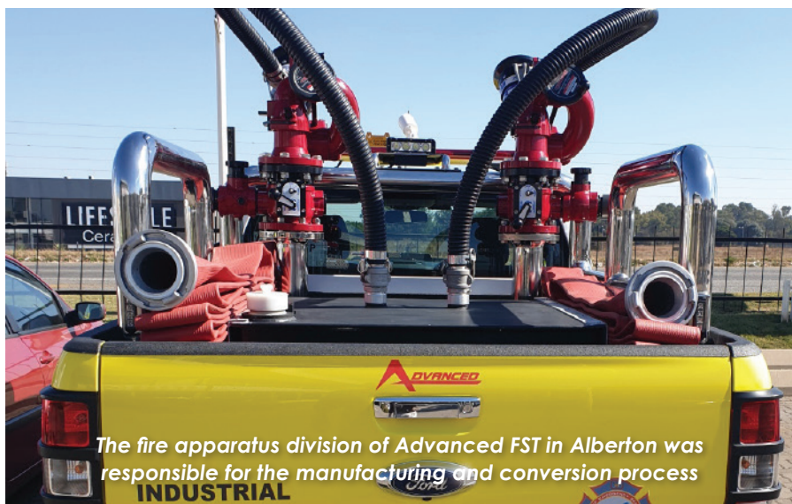
Two TFX Crossfire monitors has been fitted with a TFX Master Foam self-inducing nozzle
